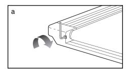
b. If the walking belt has shifted to the right, first remove the key and UNPLUG THE POWER CORD. Using the allen wrench, turn the left rear roller adjustment bolt counterclockwise 1/4 of a turn. Plug in the power cord, insert the key and run the treadmill for a few minutes. Repeat until the walking belt is centered.
